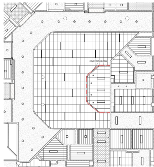
2 TYPICAL DAYROOM-1ST FLOOR RCP SCALE: 1/8"=1'-0"
